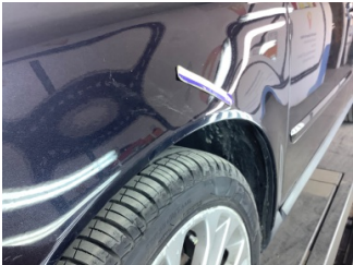
Çamurluk, sol, Çamurluk, sol > Ezik
